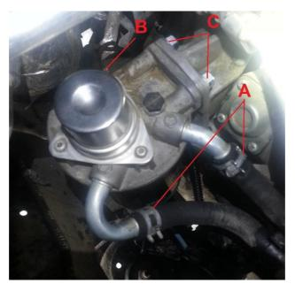
5: Unplug fuel heater wire (B) and remove T20 Torx screw (B) holding the ground terminal to the filter head. Retain the screw for reassembly.
